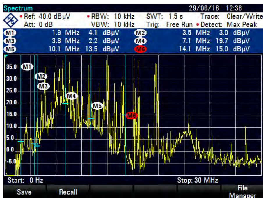
Screen2224 0 - 30 MHz, 14 MHz wire dipole 10 kHz RBW
