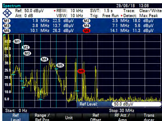
Screen2225, 0 - 30 MHz, current on dropwire 'A'
