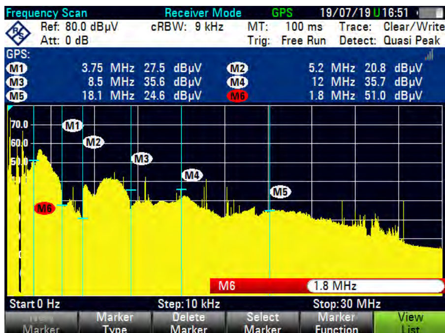
Trace0850, 0 - 30 MHz, 10 kHz step, 9 kHz RBW, QP Detector
