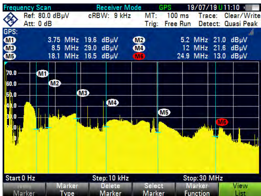
Trace0843, 0 - 30 MHz, 10 kHz step, 9 kHz RBW, QP Detector
