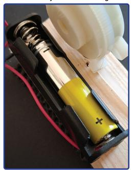
Fit the battery and ensure the polarity is correct. The black negative flat end should be towards the spring and the positive end to the red wire.
