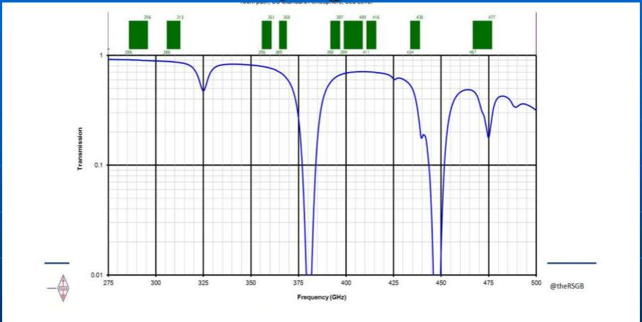
Although the oxygen losses are very low there is still up to 1dB extra path loss per km due to water vapour
