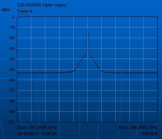
16GHz x6 mult. +9dBm @ 96GHz, then x3 to 288GHz
