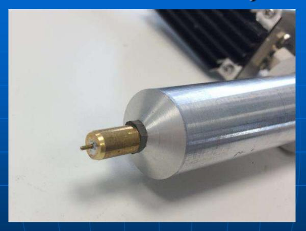
Note the tiny hole for the circular waveguide is 0.25mm and cuts off at below 704 GHz
