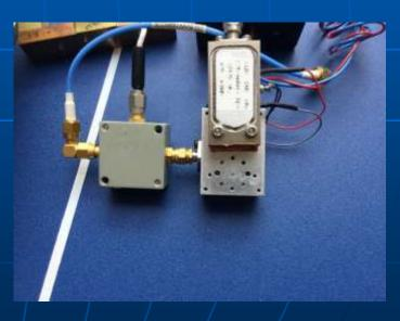
Sub-harmonic mixer used at 241 GHz with 432 MHz IF will work at 288 GHz with 47 GHz IF.
