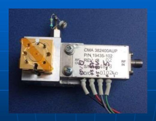
Tripler 220-330GHz, here 241GHz CMA to 40G, x2 80GHz Output ~150uW @ 241GHz (for 288 32-96-288)
