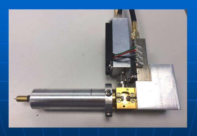
The mixer assembly mounted at the focus of the dish
