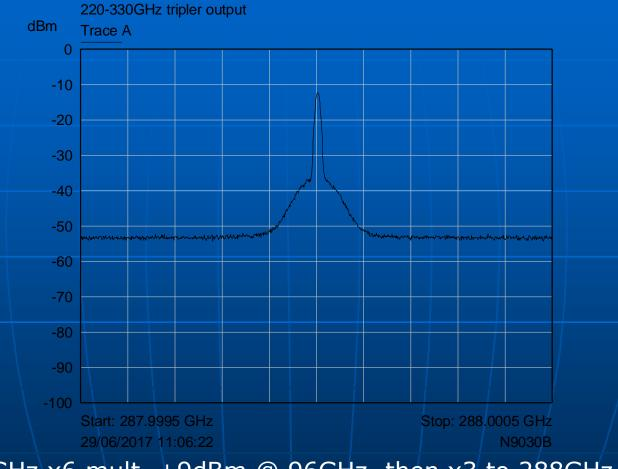
16GHz x6 mult. +9dBm @ 96GHz, then x3 to 288GHz
