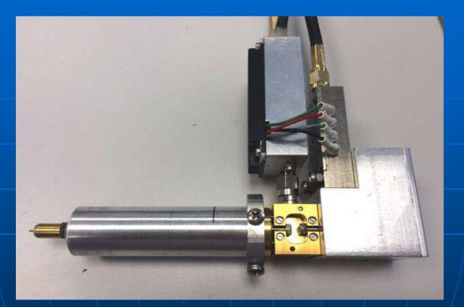
The mixer assembly mounted at the focus of the dish
