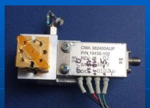
Tripler 220-330GHz, here 241GHz CMA to 40G, x2 80GHz Output ~150uW @ 241GHz (for 288 32-96-288)
