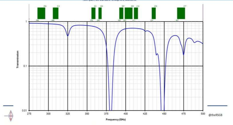
Although the oxygen losses are very low there is still up to 1dB extra path loss per km due to water vapour
