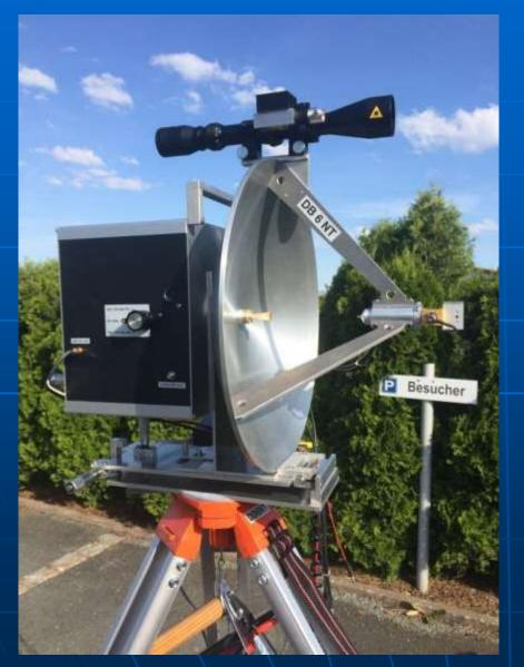
Note that in both cases (411 & 725 GHz) the antennas could be either metal or silvered glass paraboloids. As we are quasioptical we could also use lenses to provide gain
