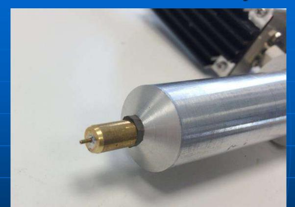
Note the tiny hole for the circular waveguide is 0.25mm and cuts off at below 704 GHz
