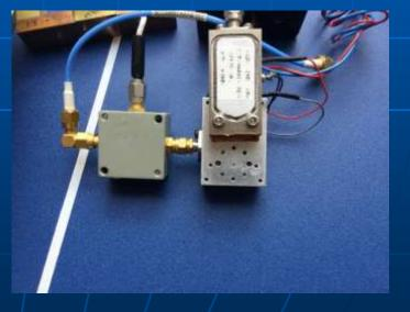
Sub-harmonic mixer used at 241 GHz with 432 MHz IF will work at 288 GHz with 47 GHz IF. Possibility to make dual band 241/288 GHz transverter.. SSB signal using mixing already received at 7 km on 241 GHz. Potential for aligning / QSO on 241 then switching to 288 GHz
