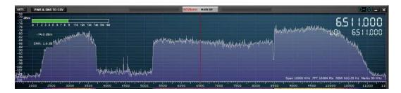
Finally, the RSGB has developed a software tool called Lelantos, written by Dr Martin Sach G8KDF, a member of the EMC Committee, which can detect VDSL signals. This software, when fed with a spectrum recording made from an SDR receiver, uses the synchronisation signals buried within the VDSL spectrum to positively identify whether or not an interfering signal is VDSL. Further information can be found in RadCom November 2018 and in EMC leaflet number 17.
