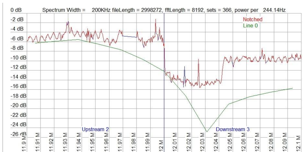
Figure 13. Expanded Lelantos spectrum display showing the 12MHz VDSL guard band
