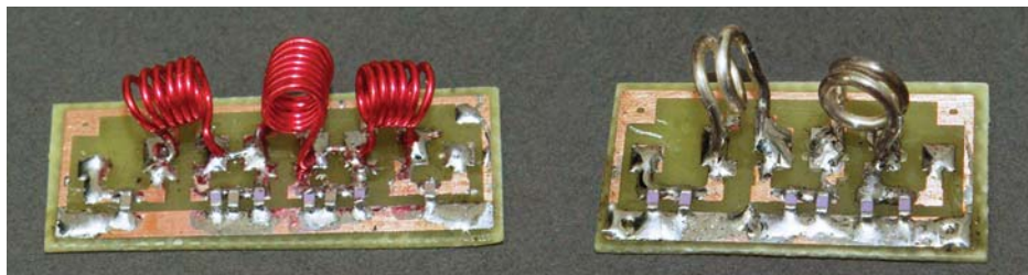
PHOTO 1: The two breadboard filters, constructed using SMT capacitors on a generic filter PCB.
