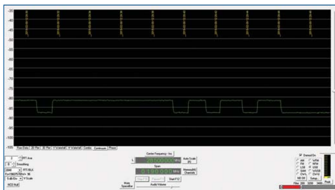
FIGURE 1: Screen capture of Spectravue in continuum mode used for noise level measurement. Noise source driving a Microwave Modules converter feeding the SDR-IQ receiver. Y factor = 6.5dB.
