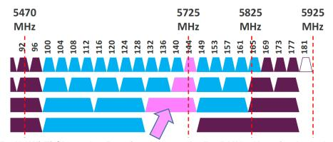
5 GHz Wi-Fi Channels: Restricted due to the 5725 MHz allocation boundary
