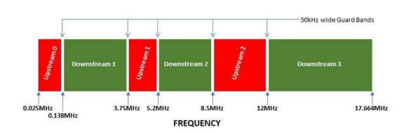
The best ones to investigate are at 5.2MHz, 8.5MHz and 12MHz. If the background noise decreases on one side of the guard-band frequency and then rises again on the other side, then this would indicate the presence of VDSL interference. If an SDR receiver is used, then the guard-bands may be clearly seen on a spectrum display. The following diagram clearly shows the VDSL spectrum with guard-bands at 8.5MHz and 12MHz.
