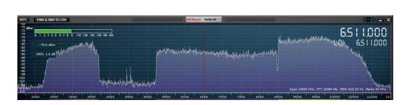
• Finally, the RSGB has developed a software tool called Lelantos, written by Dr Martin Sach G8KDF, chairman of the EMC Committee, which can detect VDSL signals. This software, when fed with a spectrum recording made from an SDR receiver, uses the synchronisation signals buried within the VDSL spectrum to positively identify whether or not an interfering signal is VDSL. Further information can be found in RadCom November 2018.
