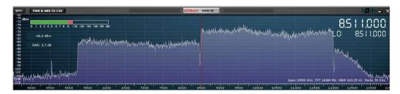
The following diagram shows an expanded example of the 8.5MHz guard-band.
