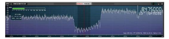
In addition, with an SDR receiver, the 4.3125kHz pattering of VDSL carriers may be observable on a waterfall display.
