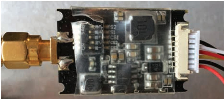
PHOTO 2: Close-up of a typical transmitter module. The DIP switches on the left set the operating channel.
