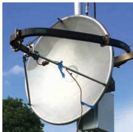
PHOTO 6: 10GHz dish with 5.6GHz dipole feed.
