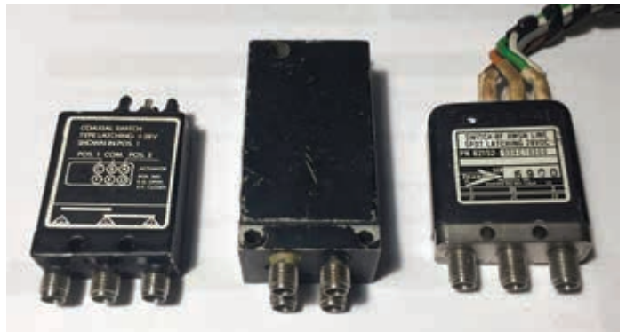
PHOTO 8: Typical suitable changeover relays. Those with four RF connectors are ‘transfer’ relays, which are also suitable for Tx/Rx changeover use.
