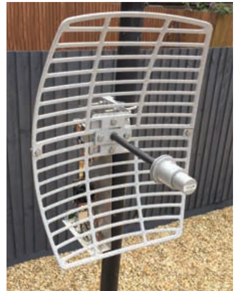
PHOTO 4: Hyperlink Technologies HG5 827G 27dBi 5.8GHz grid dish.
