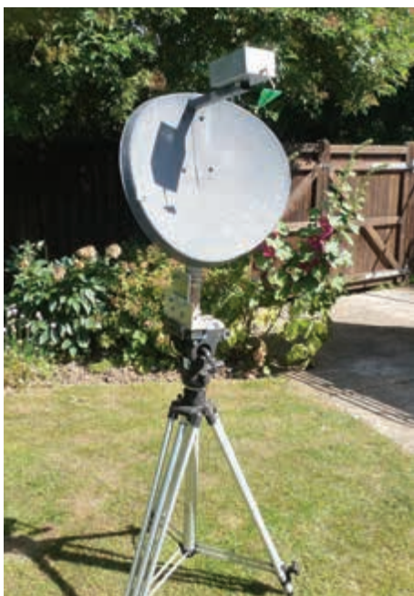
PHOTO 5: Sky dish with W1GHz log-periodic feed (the small green triangle).
