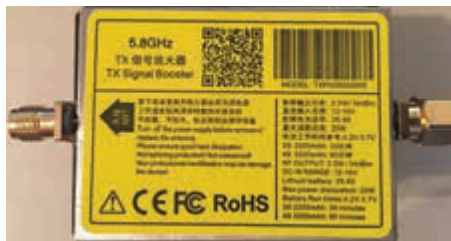
PHOTO 9: 2.5W 5.8GHz power amplifier.
