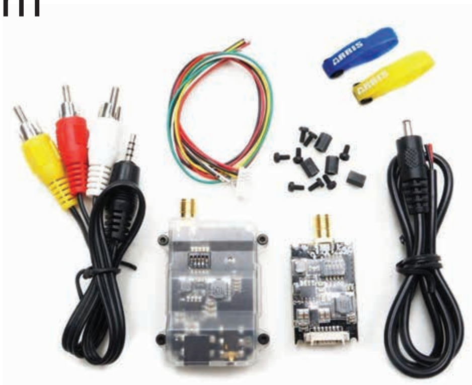
PHOTO 1: Typical 5.8GHz receiver and transmitter as purchased.
