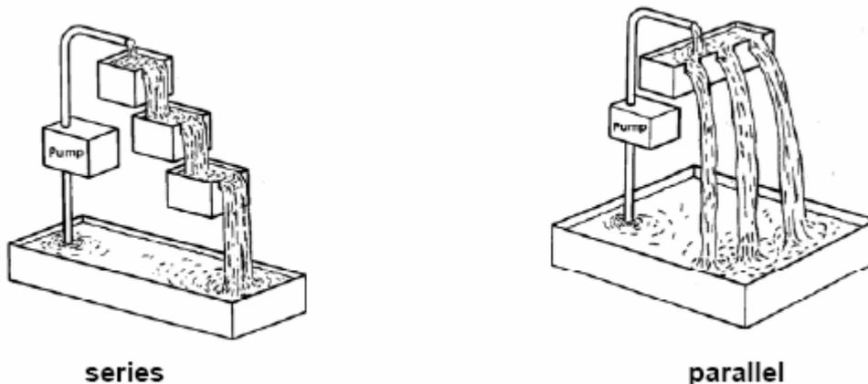
In a circuit the electric charges drop to a lower potential. In a series circuit they do this in a series of steps. In a simple parallel circuit they do so in one jump. Only some of the charges pass through any given resistor.
