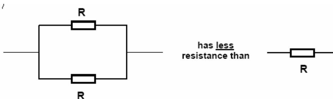
This arrangement of resistors tends to be less intuitive. It is important to stress that having resistors in parallel offers the current an alternative route so the effect of having resistors in parallel is less than having the same resistor on its own.
