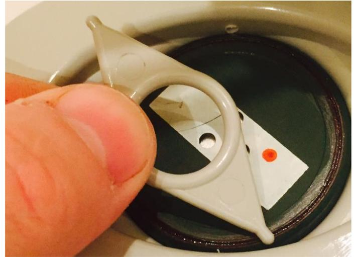
Stick a pen or similar under the plastic piece and pop it up – this allows it to be removed like so (picture to the right)
