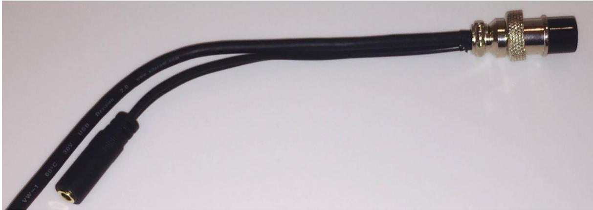
Side note: some headset may have an accessory socket. Simply cut the wires away these are not needed:
