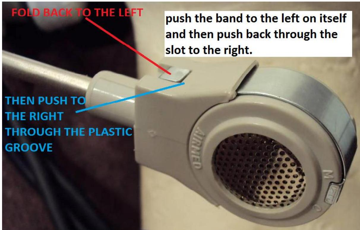
Fold the metal back on itself to the left and then push back through the plastic slot in the housing this will allow the band to become free and the circular mic element to become loose. On this version of the head set it has two wires. RED AND WHITE. The RED wire is placed inside a YELLOW sheathing and the WHITE wire is placed in a GREEN sheathing.
