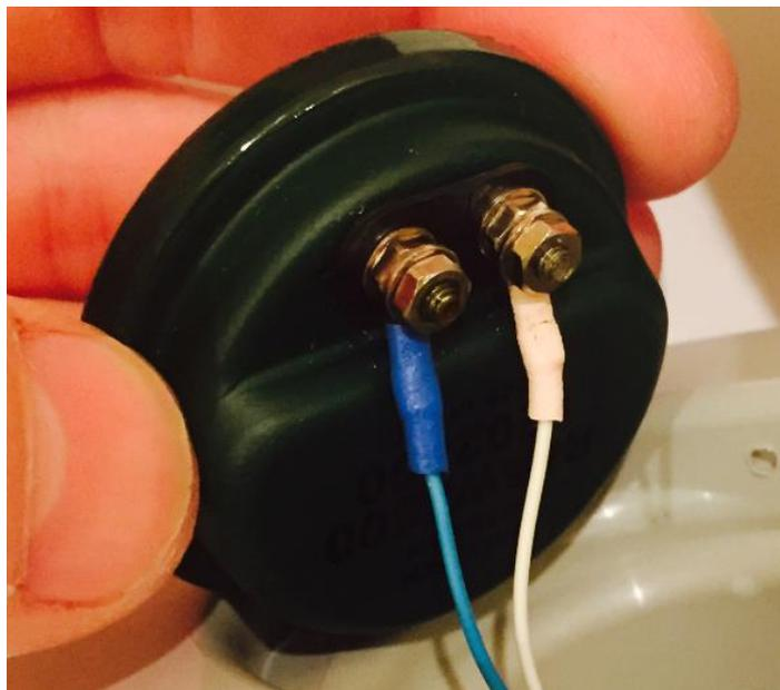
Do the same with the other speaker and note the colour of the wires.
