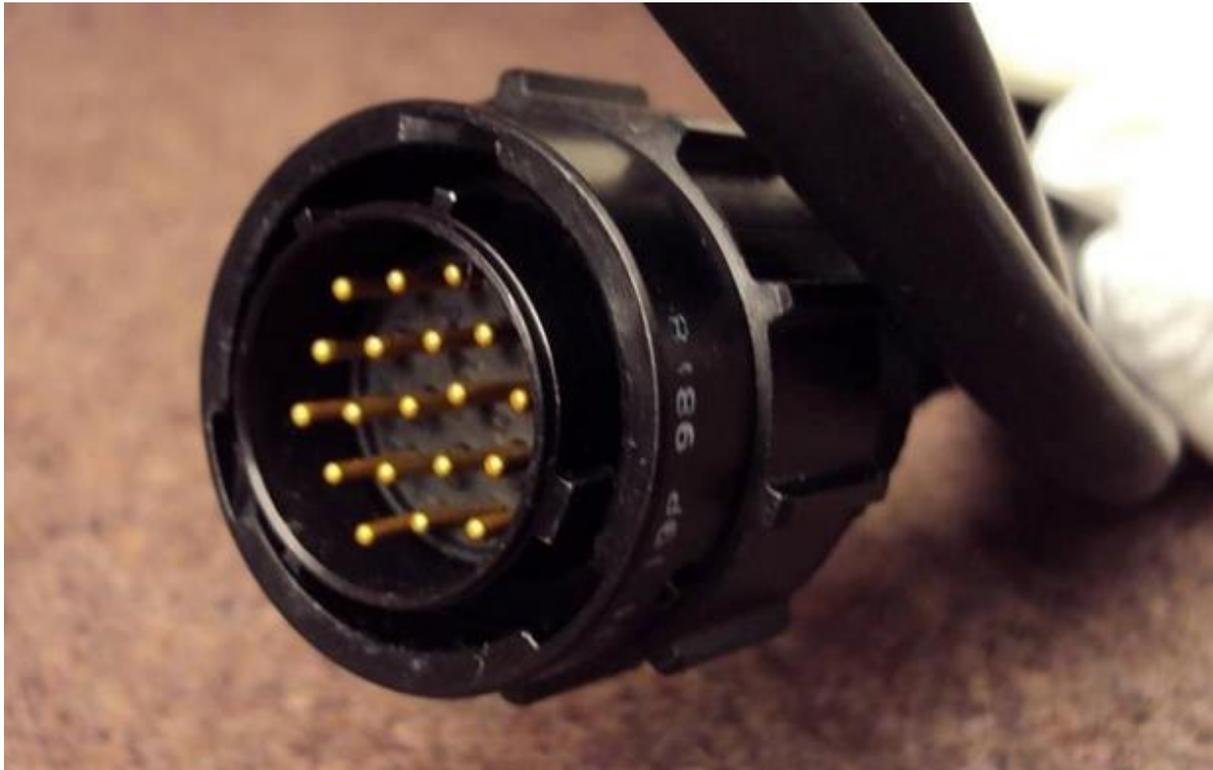
This of course will not fit any amateur radio transceiver without being re-wired. The cable on these radios are very stiff and can be awkward. They are that rigid if you move on your seat they can rise off your head. So the best option is to rewire with a new cable. Shielded USB cable will do the trick for this and then connect it to plug that will fit your transceiver such as an 8 pin plug:
