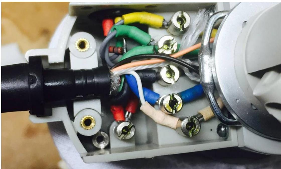
Un-screw these terminal posts and remove the ring connectors which are connected to the black cable. This will allow you to take the cable out of the housing. It's a good idea to keep the black hood.
