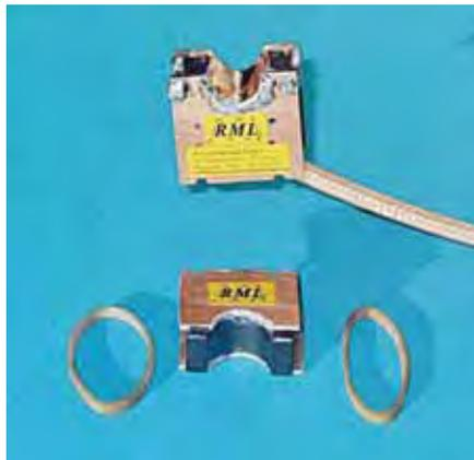
**PHOTO 3:** G3SBA's wide-band current transformer, shown disassembled. This view shows how the 5-turn secondary winding on the lower half-core is shielded with copper foil and PCB laminate. Once assembled round the cable-on-test the two halves are held tightly together by the elastic bands.
