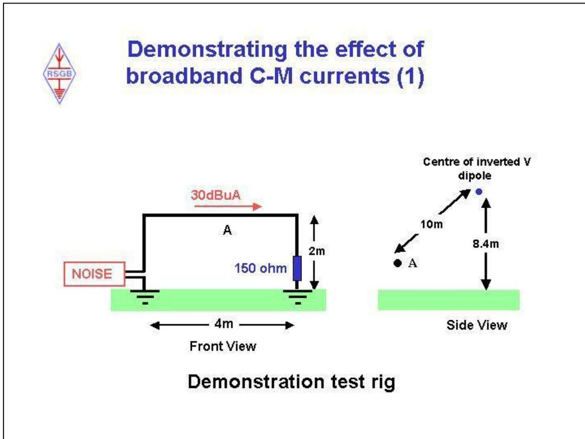
The intention of slides 5 and 6 is to draw attention to the fact that, where conductor deployment leads to a significant proportion of the energy being radiated, the levels of common-mode current permitted by product standards such as CISPR 22 would give rise to severe interference to small-signal services.
