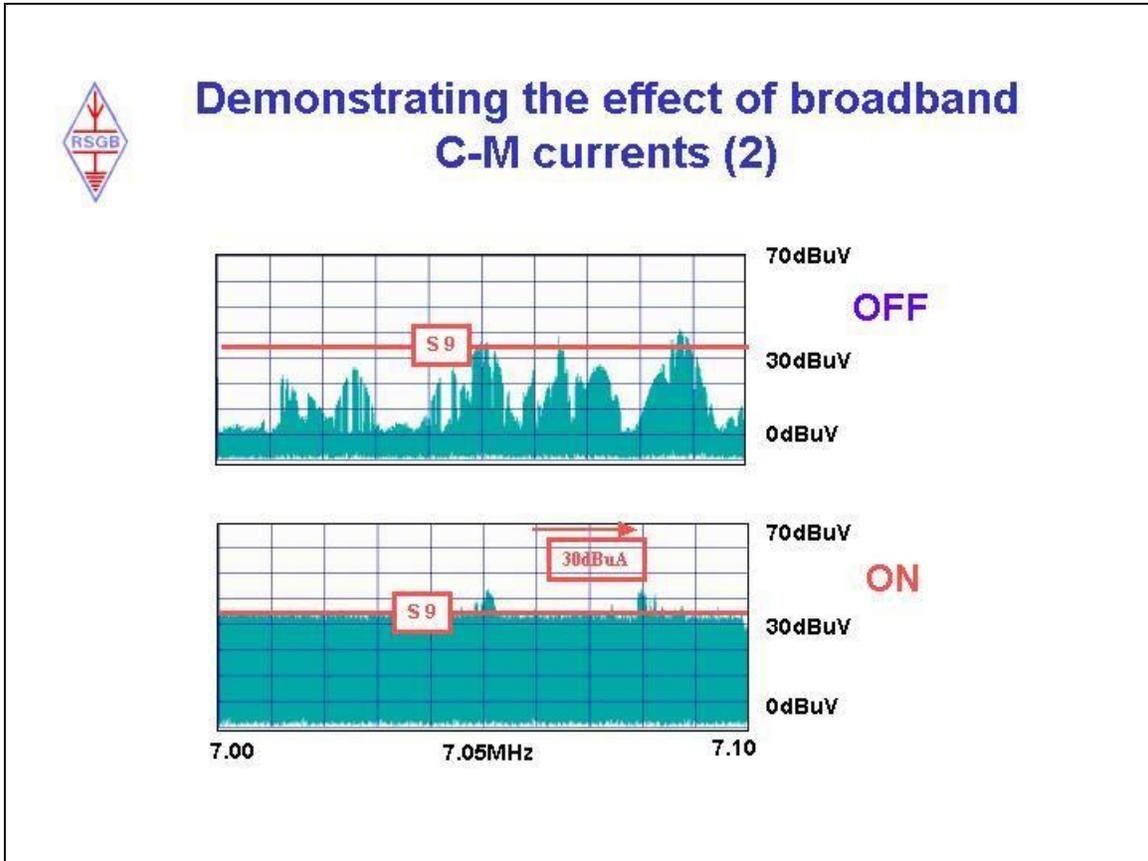
The vertical axis is the signal from the inverted V dipole. The baseline of the plot is the instrument noise floor not the ambient noise (see slide 2 above).
