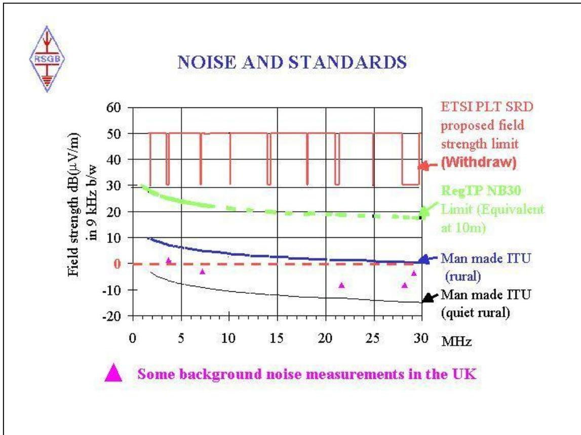
Slide 3 illustrates the significance of ambient noise levels and proposed standards in the HF band. The NB30 limits have been calculated for a distance of 10m from the original levels at 3m. The ETSI PLT SRD limit was from a draft document which has since been withdrawn. It is included as an indication of the magnitude of the regulatory problems.
