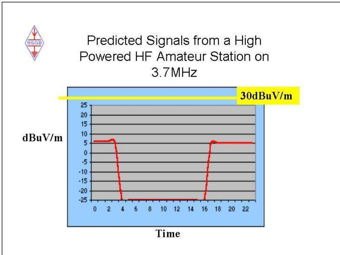
The basic slide is taken from the predictions of signal strength in the UK for signals from the "Dexpedition" station on the Comoro Islands. This would be running relatively high power to a good antenna. A 30dBuV/m line was added because a 30dBuV/m limit for the amateur bands was under discussion at the time. The proposal which gave rise to this has since been withdrawn.
