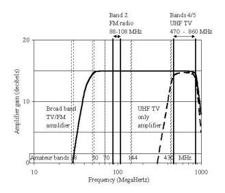
Fig. 1. The typical response of two types of TV distribution amplifier.
